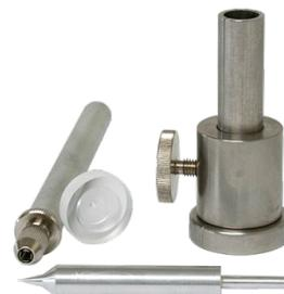
Figure 3: Pharma test kit, Micro Cone, acc. to Klein
